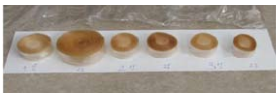
Figure 5. LLDPE based film rolls: 1% and 2%; PP based film rolls: 1 and 2%; mixed based film rolls: 1 and 2%
